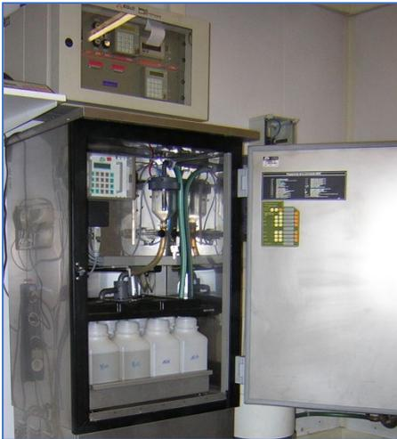
This fully programmable unit enables pre-determined volumes of water to be collected over a fixed time period and frequency.
