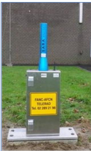
**Gamma spectrometry stations** (about 65) for measuring the ambient gamma radioactivity and the gamma radioactivity of certain radionuclides (10 predefined nuclides), are distributed on the fences around all nuclear sites and in the agglomerations (~ 5 km around the site) of the Nuclear powerplants Doel and Tihange. Photographs show a station in its environment.
