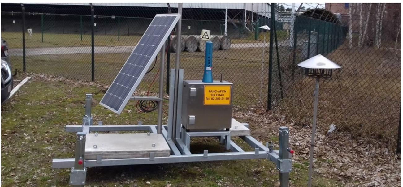
The **aerosol stations** (ZnS detector), of which there are 7 for measuring the radioactivity of dusts suspended in the air (aerosols and fine particles), which determine the total alpha and total beta radioactivity.
