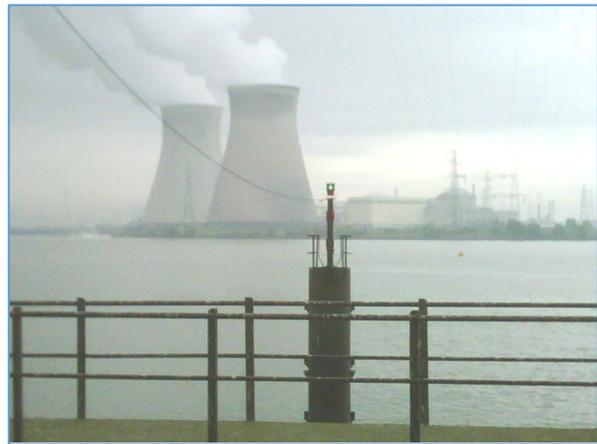
TELERAD also has 6 stations (BCI) in the release channels of the nuclear power plants which continuously measure the gamma radioactivity of the releases: one in the release channel and one upstream/downstream of the nuclear power plant of Doel and three in the release channels of the nuclear power plant of Tihange. These stations allow to monitor the liquid discharges from the electricity producers with close attention.
