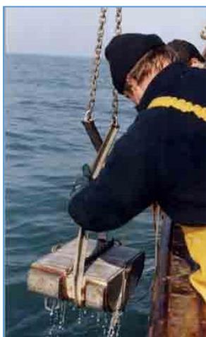
As soon as the jaws touch the bottom, the spring which keeps the jaws open is released. Before returning to the surface, the jaws close and trap a quantity of sand or sediment from the sea bed.
